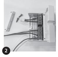
Prepare cables and make connections to screw terminals.
