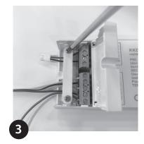
Check all connections are correctly made and secure.
