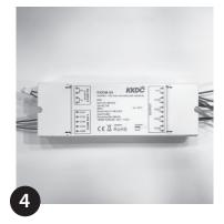
Close terminal block covers and fix with suitable screws. Do not over tighten.
